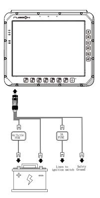
**Fuse Requirements** Fuses\* are required in connecting the power cable and battery in series and add 3A fuse in ACC/ignition line to avoid the risks of wire damage and vehicle burning. For detailed power wiring diagram, please refer to the Powering the System section of Chapter 4 in VULCAN X's user manual.
