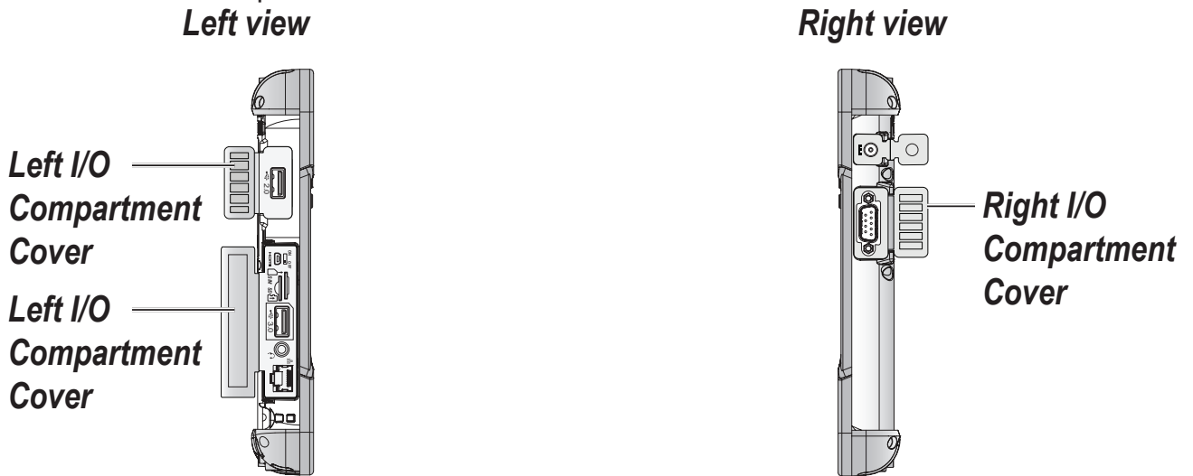
Figure 22. Side View: Locating the I/O Compartment Cover
