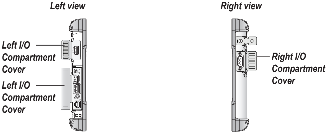
Figure 25. Side View: Locating the I/O Compartment Cover
