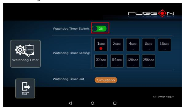
If you'd like to test if watchdog timer is enabled and working, please click on the "simulation" icon. The "simulation" is to simulate the system on hang and reboot it after the set time frame.
