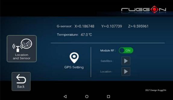
Module RF: to enable or disable the GPS receiving function.
