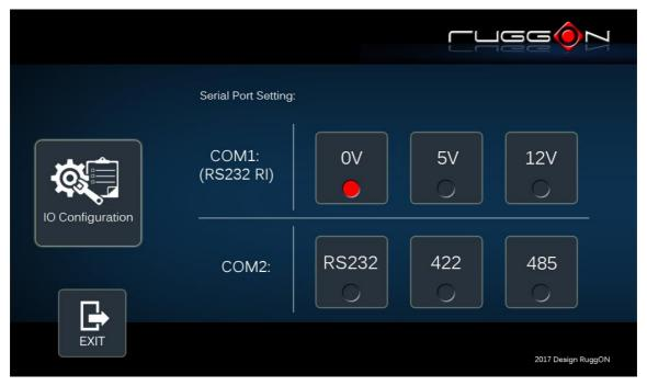
If you don't need the power output, just select 0V output to avoid the equipment damage. Please note if system power source is from backup battery (no DC input available), COM1 will stop supplying the power output.
