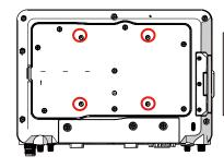
The MT7000 supports a standard VESA version MIS-D, 75, C (75mm distance quadrate order, M5 thread, deepness 6mm) with four mounting holes on the back side of the device.
