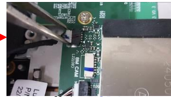
Tear off the PCBA Right MIC BOARD and Wire
