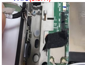
Take off the Camera board _front PCBA and Wire(S.S.T.)
