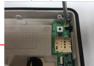
Separate the PCBA Dual SIM/Sensors Board(S.S.T.)
