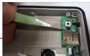
Tear off the PCBA Dual SIM/Sensors Board(S.S.T.)
