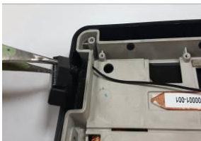
Tear off PCBA Antenna board and Wire(S.S.T.)
