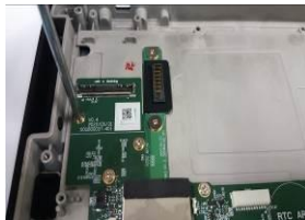
Separate the PCBA Mainboard(S.S.T.) by loosening screws
