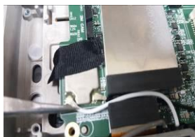
Remove the antenna cable
