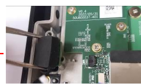
Take off the PCBA Right MIC BOARD and Wire
