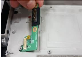
Remove the PCBA Battery charge board(S.S.T.)
